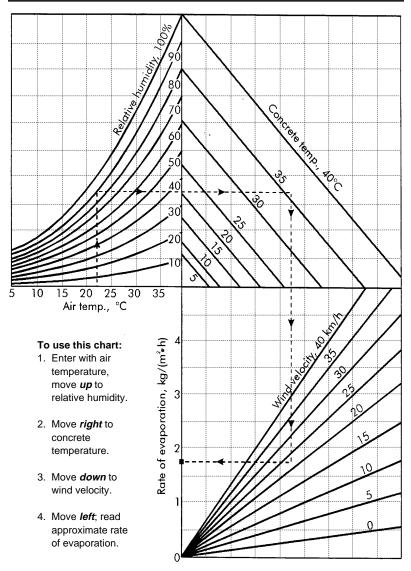
Note: Example shown by dashed lines is for an air temperature of 22.5 °C, relative humidity of 90 percent, concrete temperature of 36 °C, and wind velocity of 22.5 km/h. This results in a rate of evaporation of 1.75 kg/m²/h.
