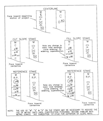
Figure 170-2.—Construction stakes.
