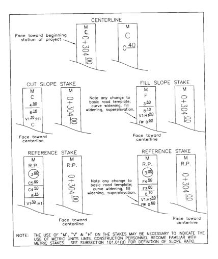
Figure 171-2.—Construction stakes.
