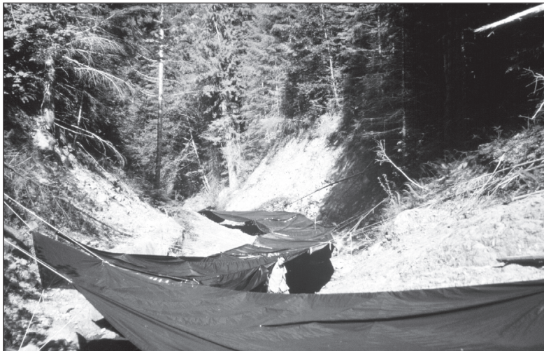
More than 1,500 square yards of black plastic sheeting and more than a mile of parachute cord was used to shade a section of stream in the central Cascades Range, Oregon.
