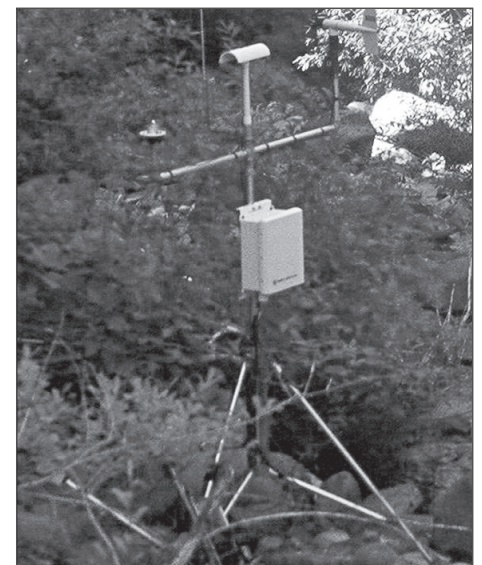
Portable climate stations, placed in several locations along the streambank, allow researchers to measure microclimatic conditions near streams
