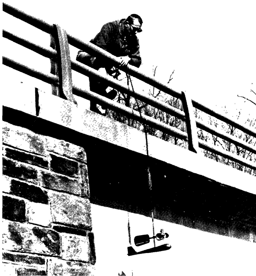
FIGURE 62.—Handline in use from a bridge.
