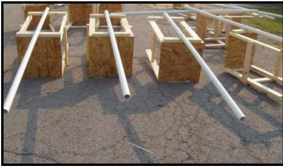
Figure 5-15. Typical preparation of sampling station supports.
