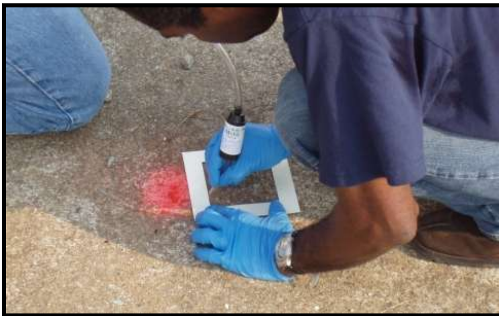
Figure 5-11. Typical surface sampling on pavement (from AACM2).
