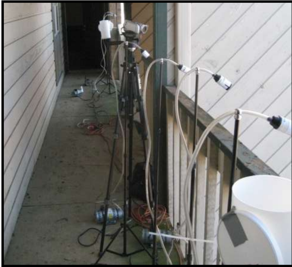
Figure 5-8. Samplers on the one of the two balconies.
