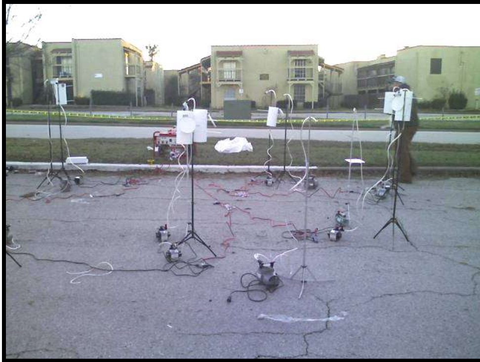
Figure 5-1. Background sampler array.
