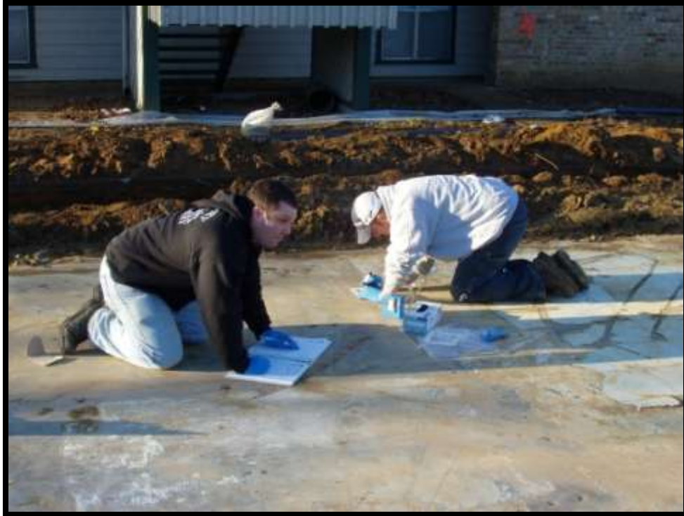
Figure 5-12. Surface sampling on concrete slab at the popcorn-ceiling building.
