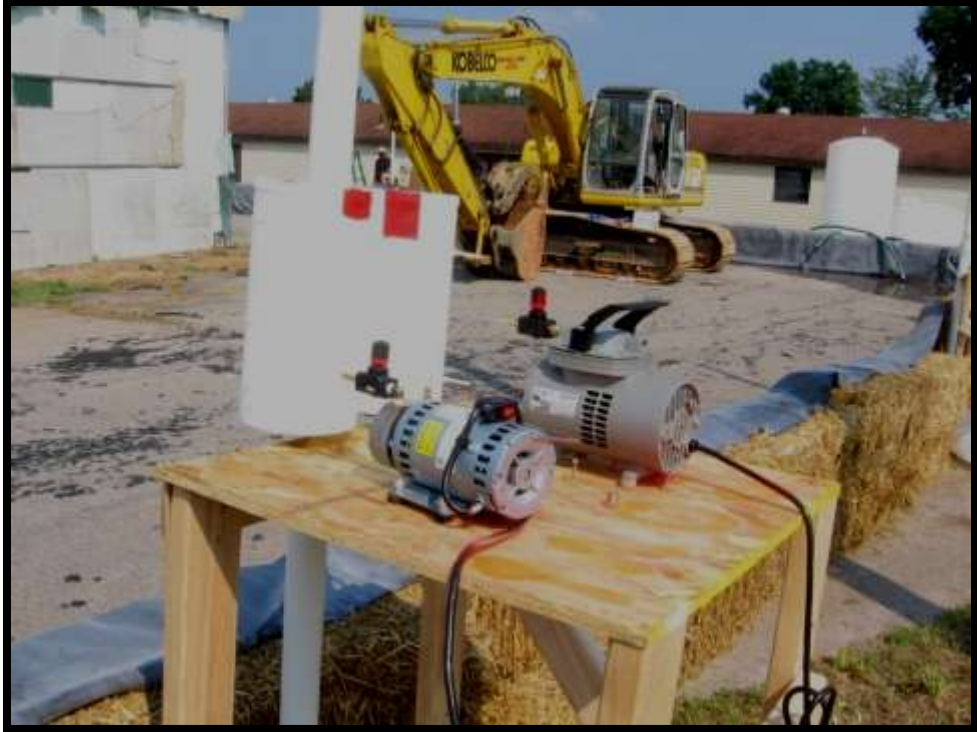
Figure 5-12. Typical sampling station.
