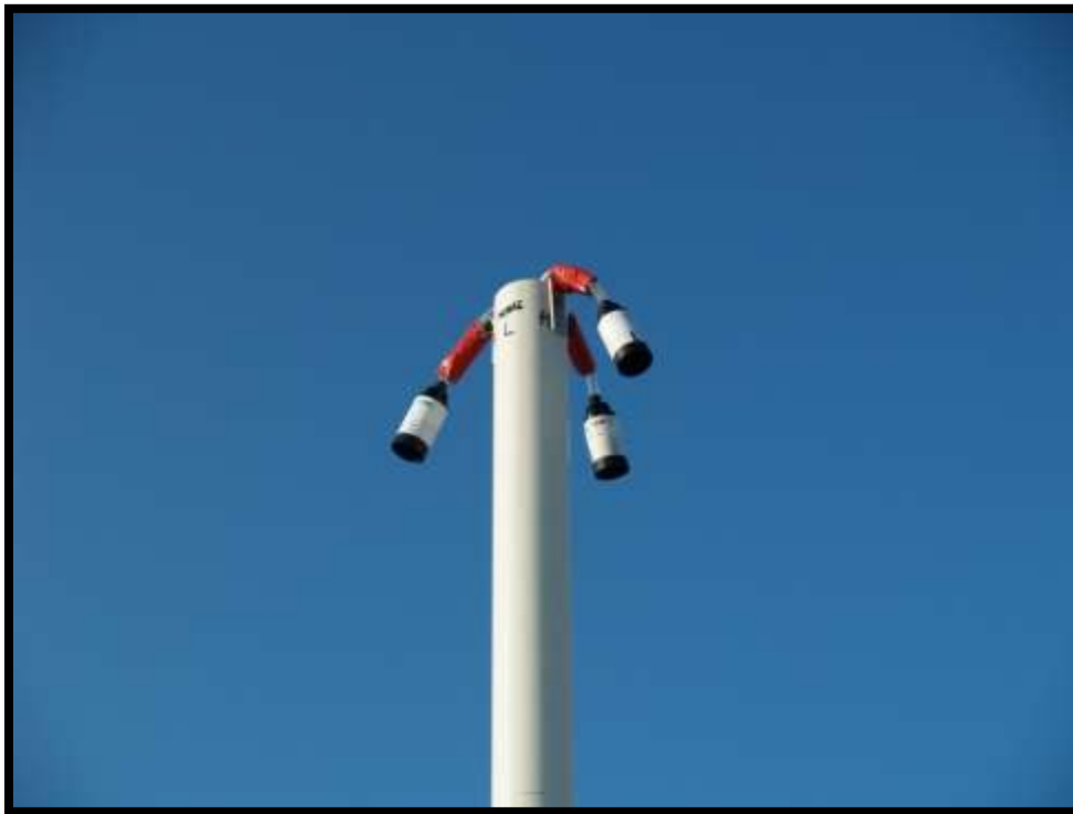
Figure 5-15. Typical samplers (high and low flow plus duplicate).
