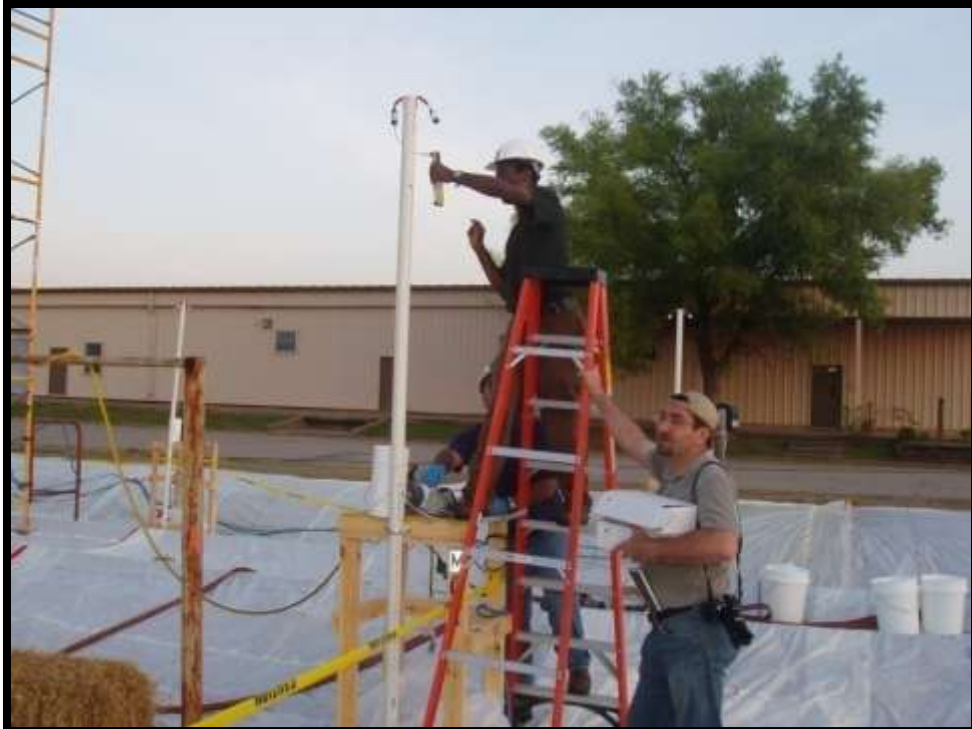
Figure 5-19. Performing periodic flow measurements on sampler arrays.
