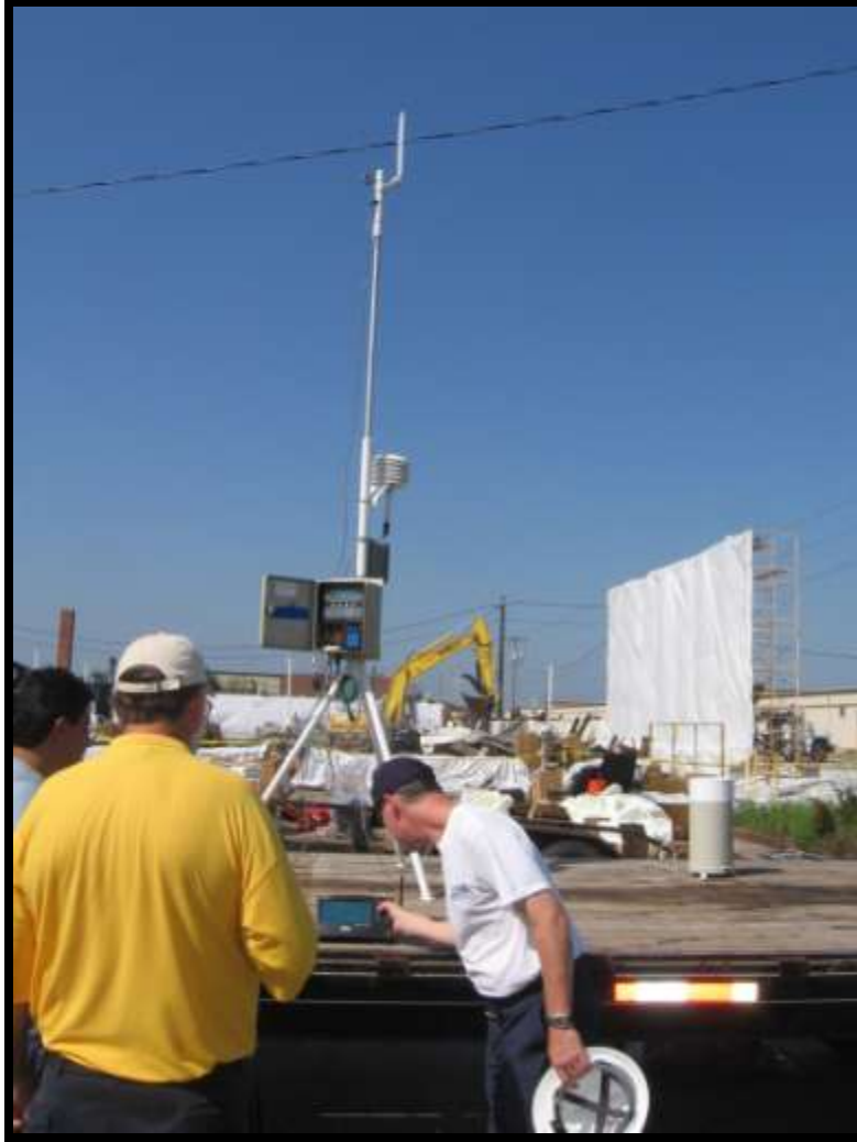
Figure 5-18. Primary meteorological sampling station.
