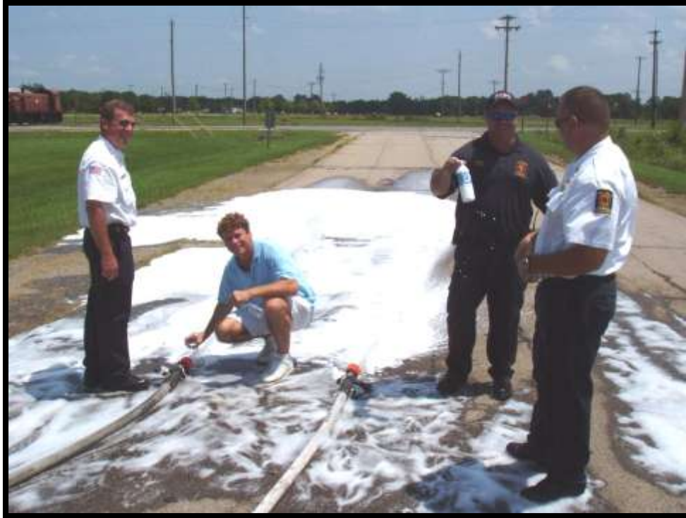
Figure 5-21. Testing amended water flows prior to the demolition.
