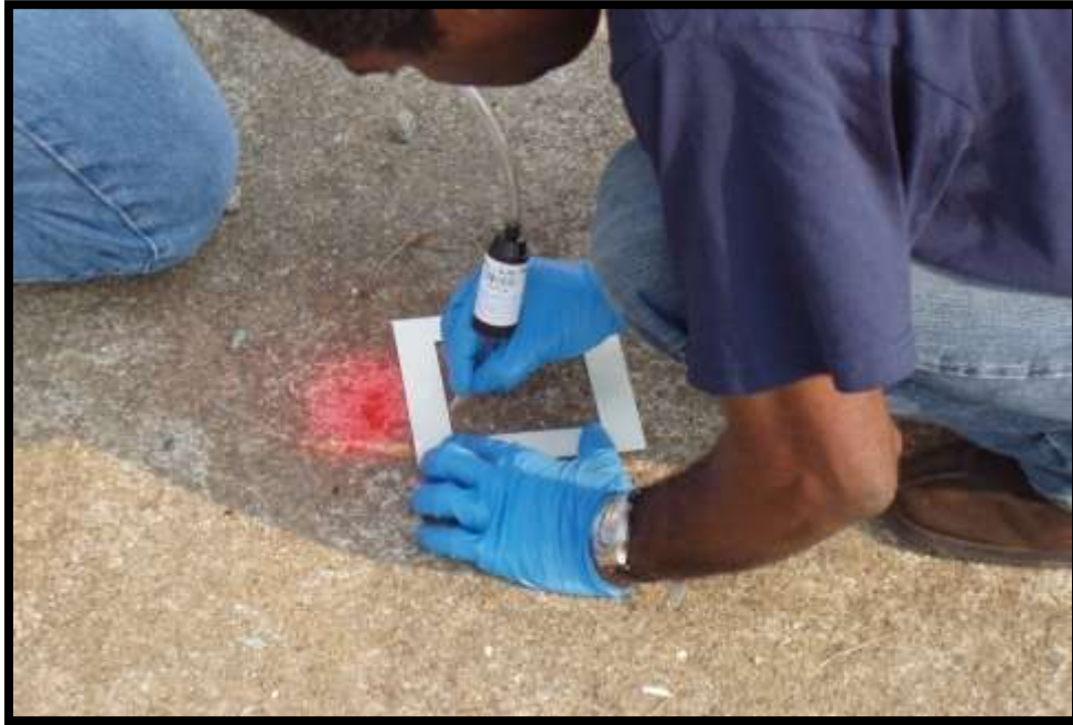
Figure 5-16. Surface sampling on pavement.
