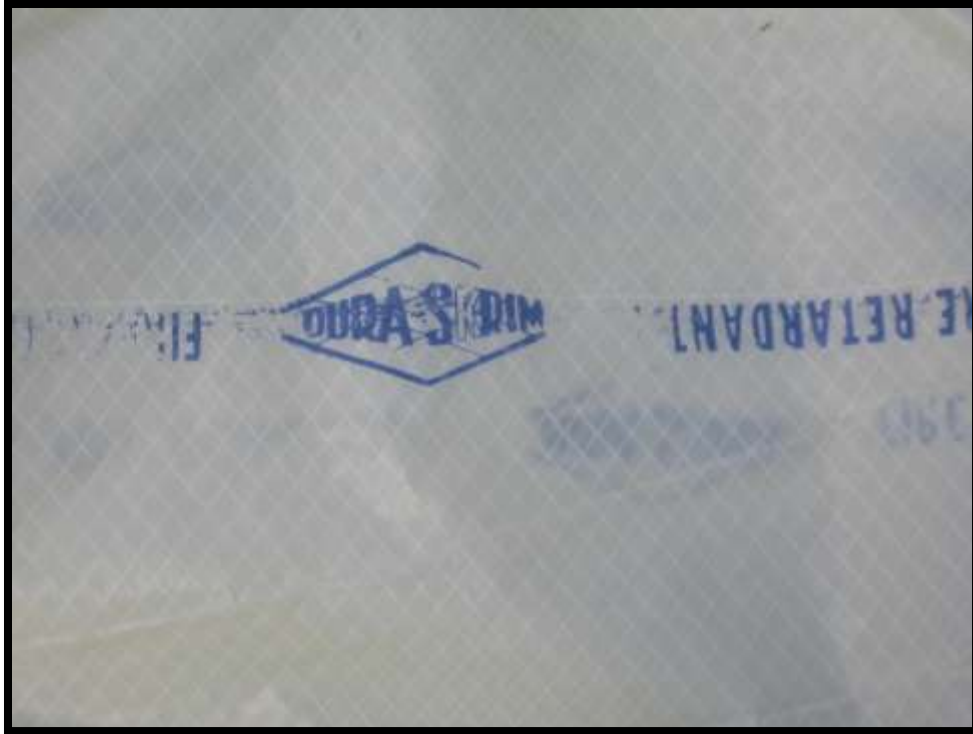
Figure 4-17. The Duraskrim fabric used for the barrier and gravel cover.
