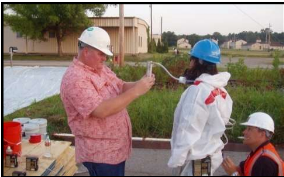
Figure 5-17. Calibrating worker breathing zone sampler.
