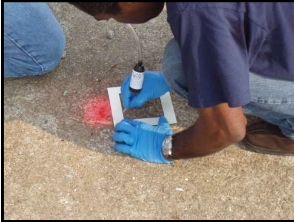
Figure 6-1. Surface sampling on pavement.
