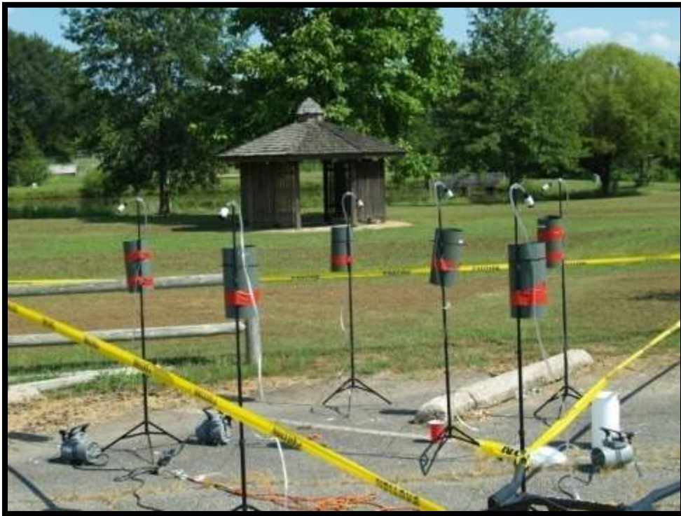
Figure 5-1. Background sampler array near the golf course.
