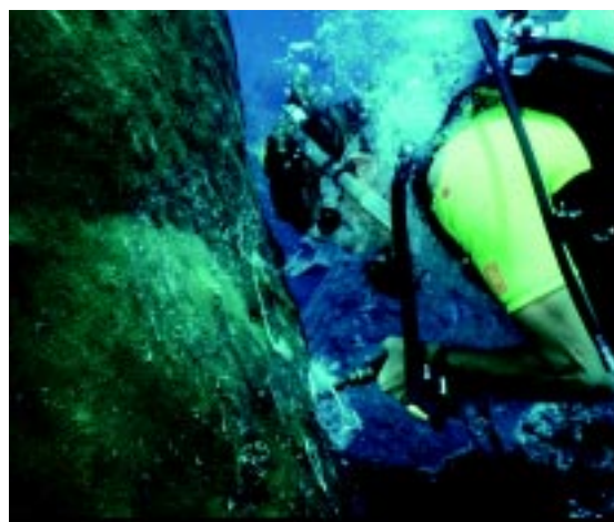
Diver removing cores from Montastraea faveolata using a pneumatic drill. (Photo: Andy Bruckner).
