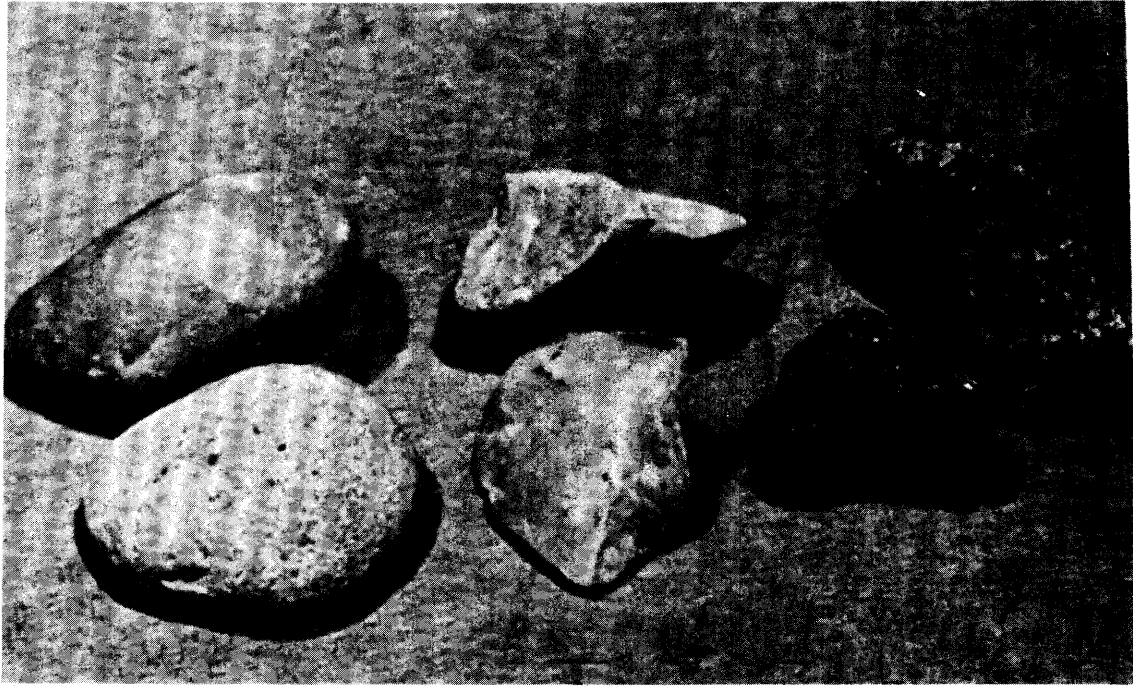
FIGURE 2.31—Aggregate of Various Shape and Surface Textures.
