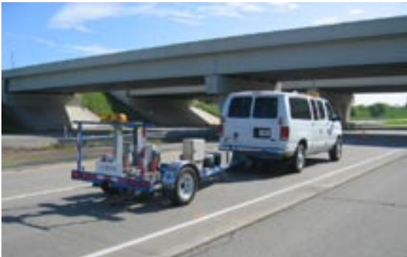
Falling-weight deflectometer testing in a multi-state investigation of the effectiveness of joint sealing (page 5).
