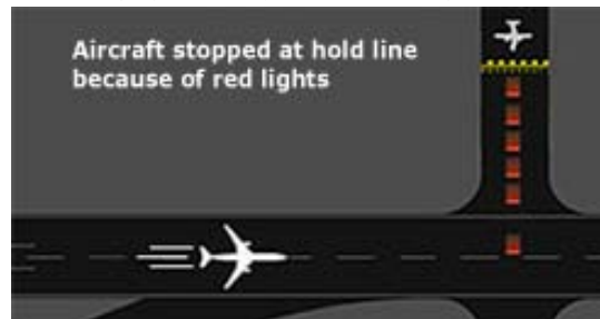
Figure 1. Illustration of RELs along a taxiway centerline (not to scale).
