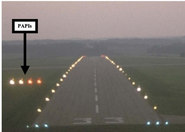
Figure 3. PAPI Light Fixture showing glide path information
