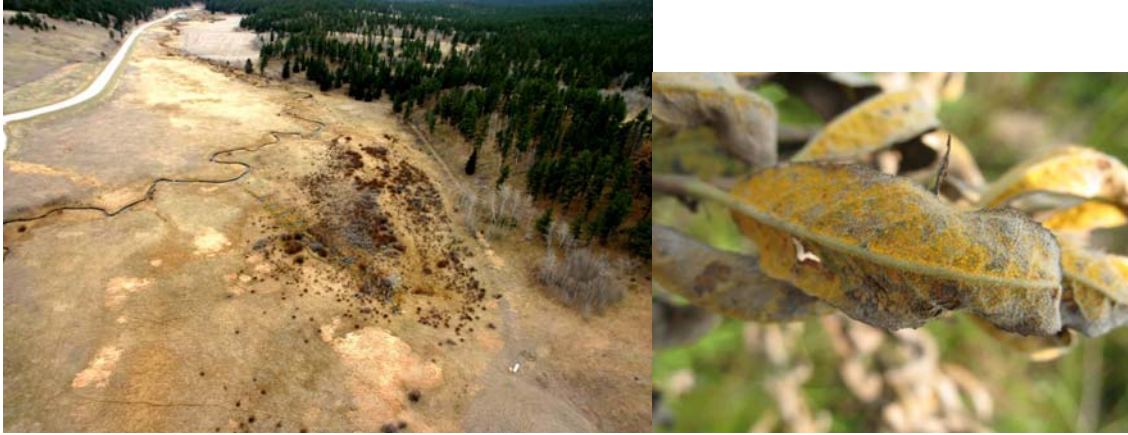
Left photo by Ken Marchand in November 2007: Aerial photo of McIntosh Fen [ Salix candida site SACA4-1]. The area in center that looks like stitching is where metal plates were installed to slow water flow out of the fen through old drainage ditch. Right photo by Cheryl Mayer on August 15, 2007: Salix candida leaf with significant cover by willow rust ( Melampsora epita ).
