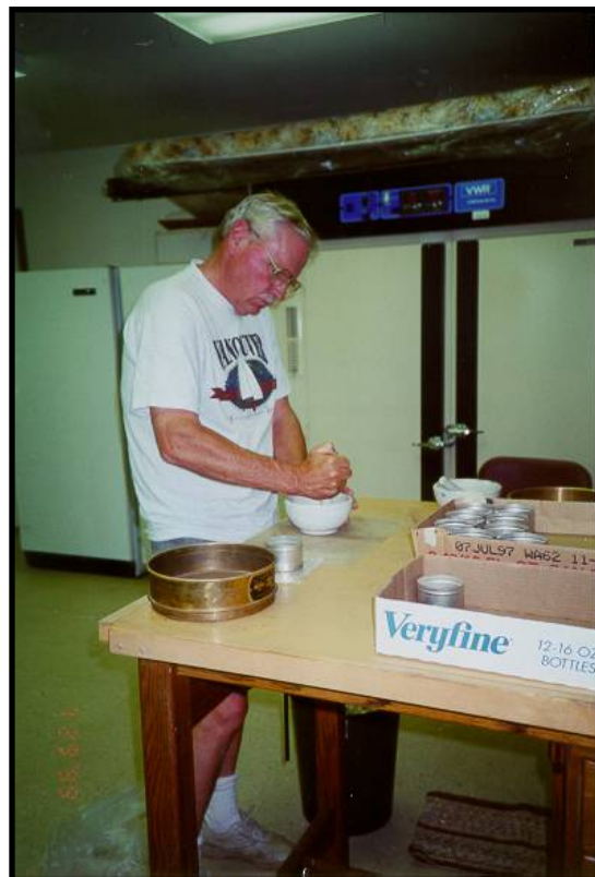
Preparing soil samples for bulk density calculations.
