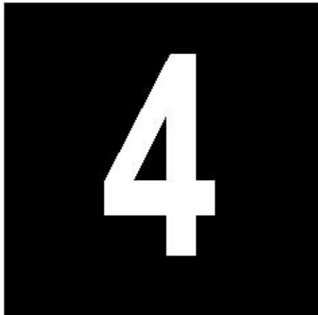
Figure 3. Runway Distance Remaining Sign (DRS). A DRS is Type L-858B, with a white legend on a black background and conforming to AC 150/5345-44, Size 4, Style 2 or 3.
