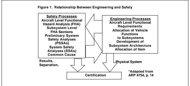
concentration on the functional breakdown, A RP 4754 recommends increased emphasis on the Common Cause Analysis (CCA) which determines how a single failure can be prevented from causing other failures.
