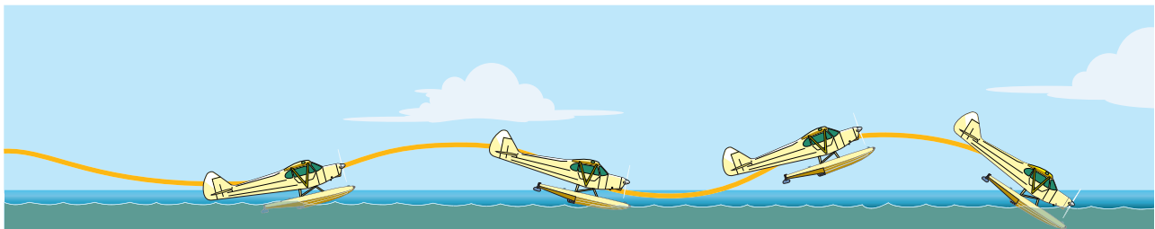
Figure 4-13. Porpoising increases in amplitude if not corrected promptly.
