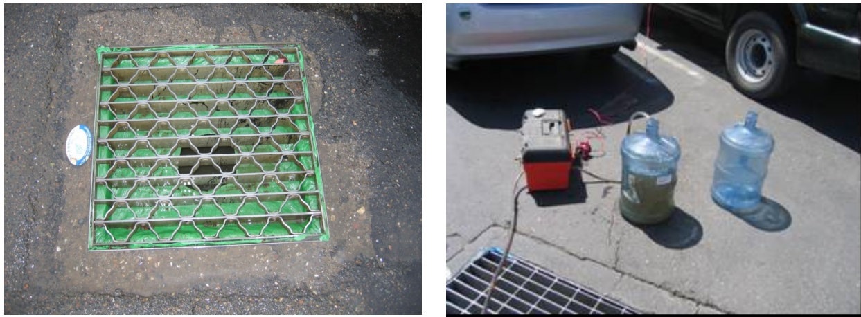
Figure 3. Storm runoff collection (manhole, pump, and 5 gal bottles)
