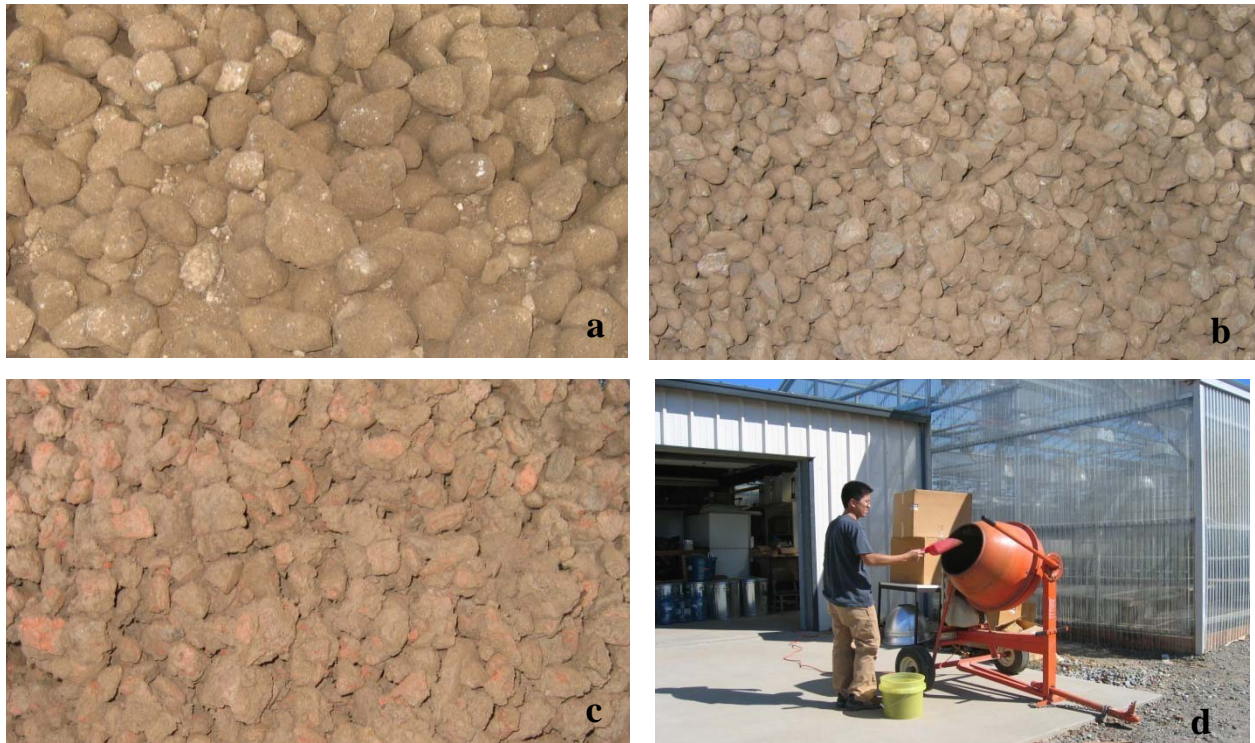
Figure 1. Engineered soils (a) CU soil. (b) CS soil. (c) DS soil. (d) Using soil mixer to make DS soil.
