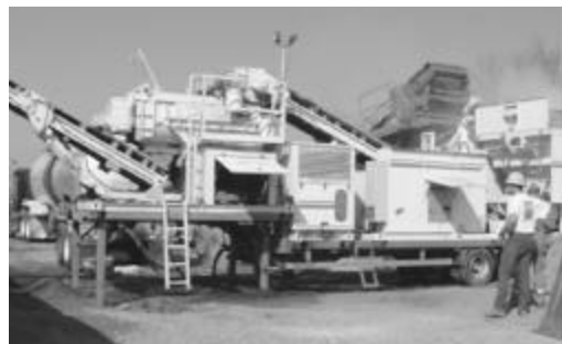
Wirtgen Pugmill mixes foamed asphalt with RAP
