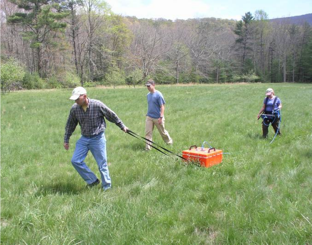
Photo 1. Ground-penetrating radar (GPR) is a geophysical method that uses radar pulses to image the subsurface. This non-destructive method uses electromagnetic radiation and detects the reflected signals from subsurface structures. Subsurface features observed in radar records need to be verified with soil borings. A GPR survey is being conducted using a 200 MHz antenna in this photo. Often, additional interpretations can be obtained by utilizing different antennas with different frequencies which consequently affect observation depths and resolution of subsurface features.
