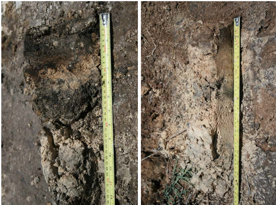
Fig. 2. The picture on the left is at the lowest point on the transect where the IRIS tube met the technical standard criteria. The picture on the right is at the highest point on the transect where no iron was removed from the upper part of the IRIS tube.
