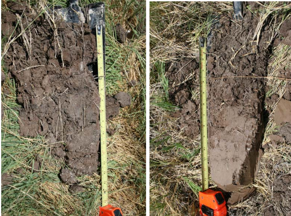
Fig. 5. The soil profile on the left is at the lowest point on the transect. It has a depleted matrix starting at 8 inches, but does not meet the depleted matrix indicator due to the 8 inches above the depleted matrix being all high chroma. The profile on the right is at a point on the transect that is definitely not wet.
