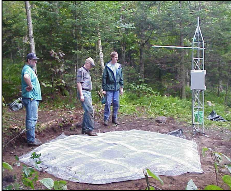
Snow pillow is filled with non-freezing liquid and is designed to measure weight and depth of snow in order to calculate snow density and water content.
