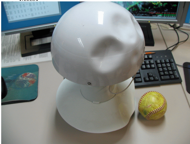
Damaged ASOS temperature housing, referenced to a softball.
