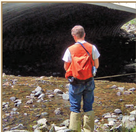
Field crew measuring stream channel conditions and biota at a recently built arch culvert.
