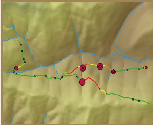
Figure 3. Estimates of fine sediment delivered to streams from road surface erosion prior to restoration treatments on the Olympic National Forest. Road segments with the highest sediment delivery rates are displayed in red and orange. Circles show locations and estimated amounts of sediment delivery. Comparable estimates were produced after road treatments to assess their effectiveness.
