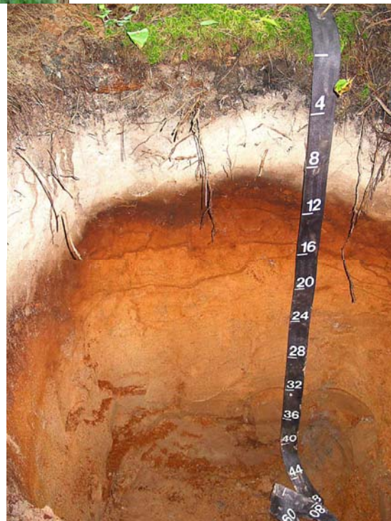
Classic podzol soil layers, showing white horizon where minerals have moved out, and the darker horizon below where the minerals accumulate.
