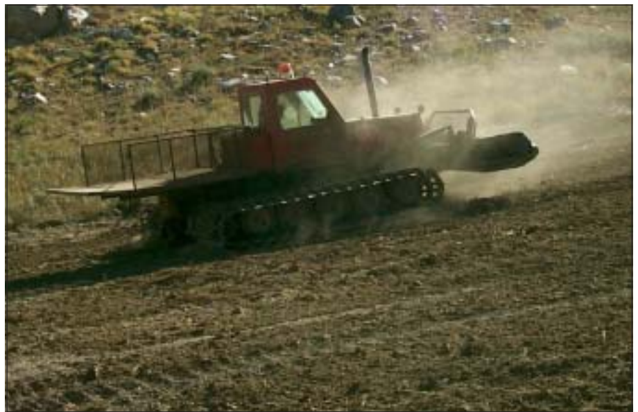
For improved seed germination, a snow cat can be used to track in and cover the seed with a thin layer of soil.
