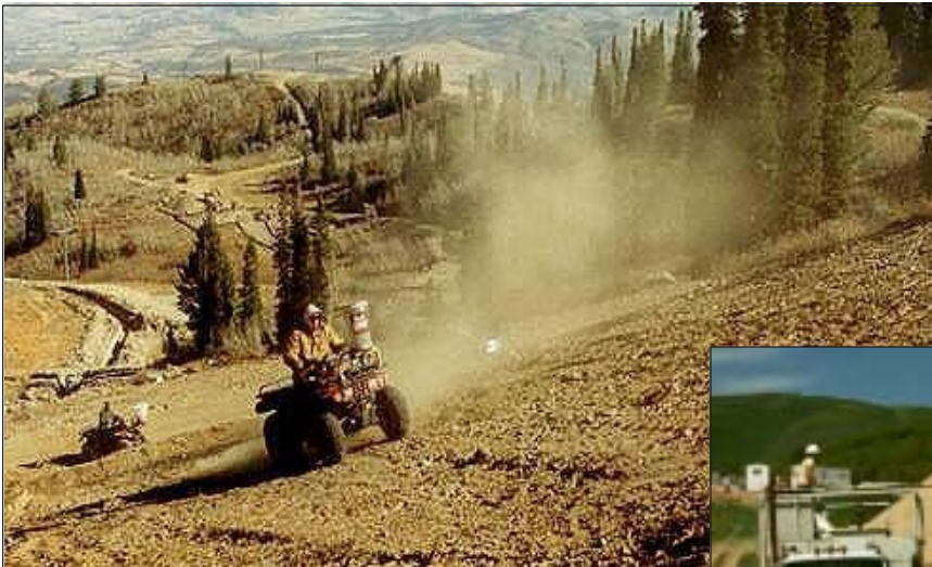
For gentle or moderate slopes, seeding equipment can be mounted on all terrain equipment to cover large and inaccessible areas.
