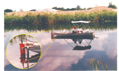
TYPICAL ADCP MEASUREMENT
