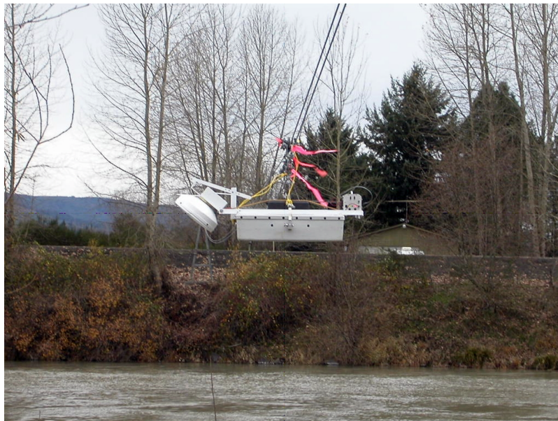
Figure 8. Continuous wave RiverScat system (antenna and control box) mounted atop a GPR antenna suspended from a cableway approximately 3–4 m above the water, across the Cowlitz River, Washington.
