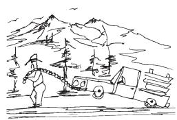
at a decided disadvantage for several reasons. Usually the reason for the tow is the towed car is not running; therefore, the defroster does not run because it is dependent on the hot water from the engine. At 20-below, trying to see through an icy windshield is not an easy thing to do. Power steering and power brakes are two other mechanical conveniences found on most cars today that won't work in a non-running vehicle.
