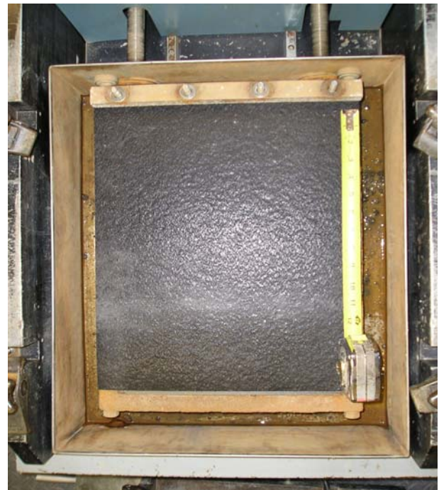
Lower box with placed geomembrane.
