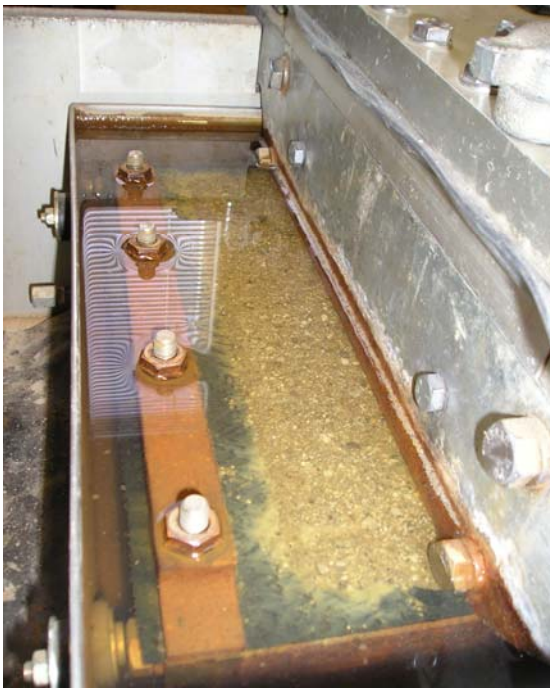
Completed test showing sand and geomembrane. Flooded box.
