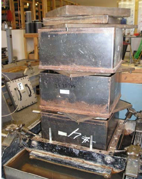
Test set up using weights for normal load.
