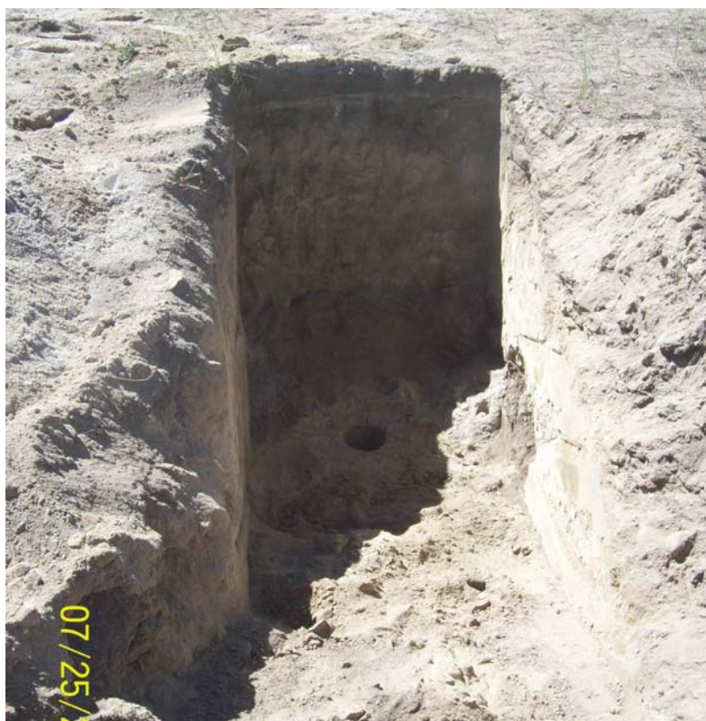
Photograph A-12. USFS – Meyers Landfill – Infiltration test pit ML-TP-02 PERC-1. Photographed: July 25, 2008
