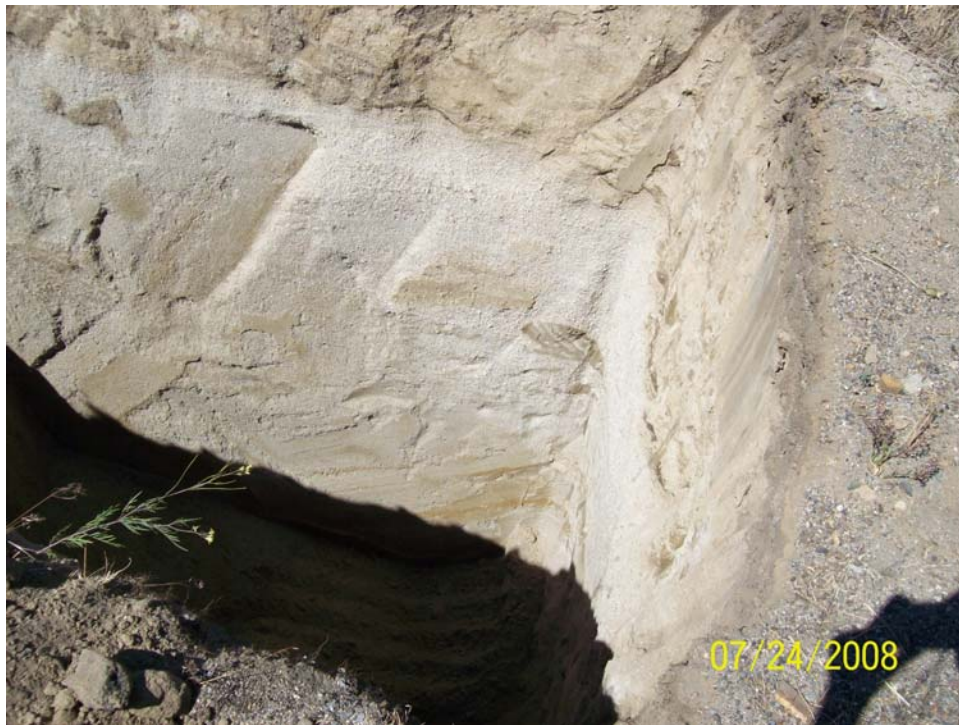
Photograph A-7. USFS – Meyers Landfill – North wall of ML-TP-01 with silty lenses visible. Photographed: July 24, 2008
