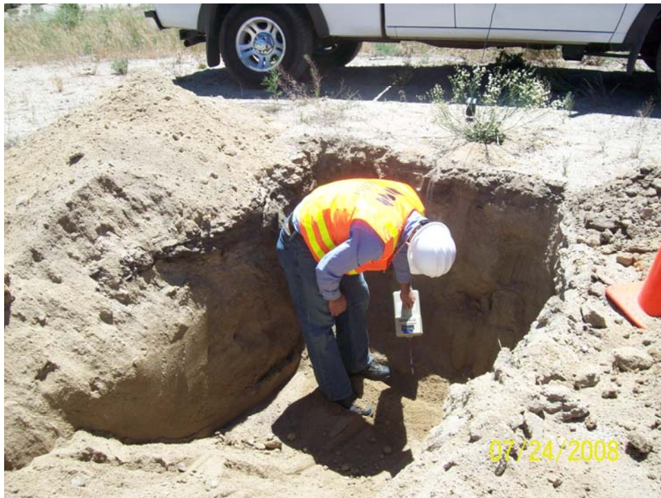
Photograph A-2. USFS – Meyers Landfill – Checking ML-TP-02 PERC-1 with the PID. Photographed: July 24, 2006
