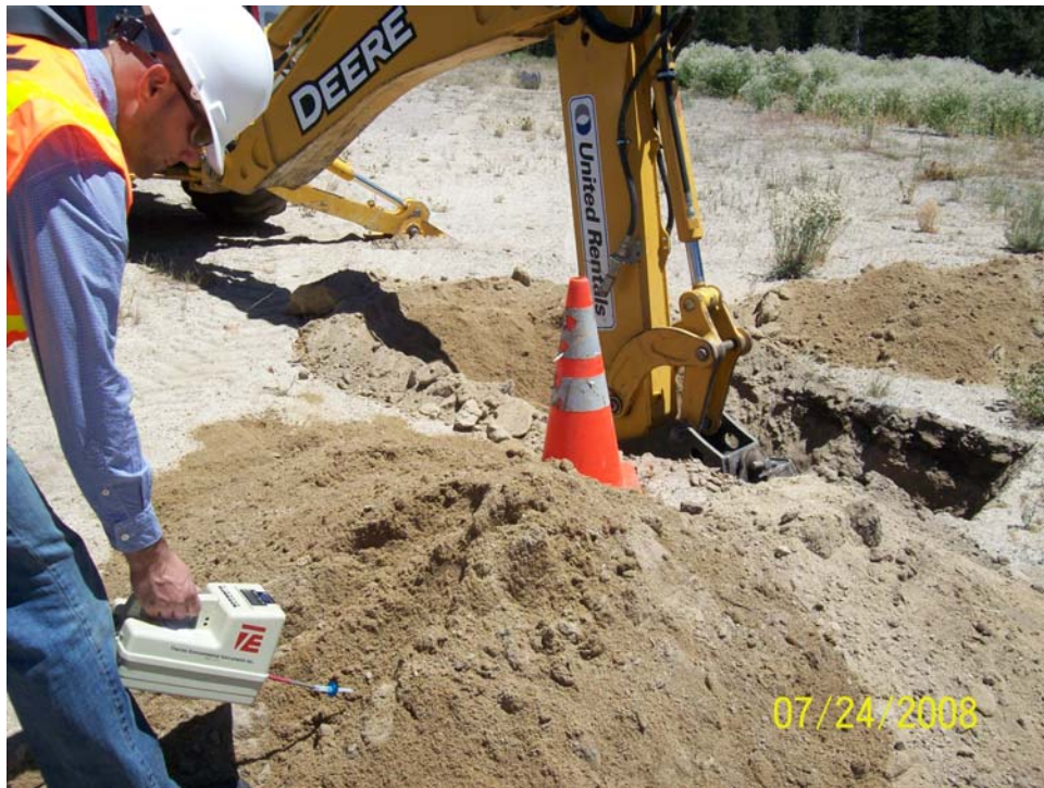
Photograph A-1: USFS – Meyers Landfill – Checking spoils from ML-TP-02 PERC-1 with the PID. Photographed: July 24, 2008
