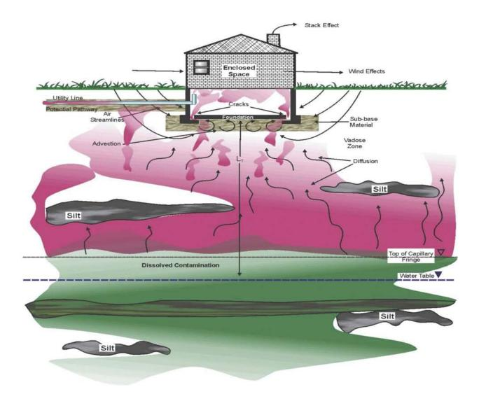
Figure B-1. Example of Conceptual Site Model cross section diagram illustrating potential subsurface vapor intrusion pathways
