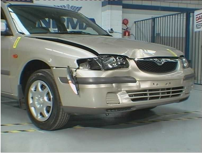
Figure 4. Typical vehicle damage in RCAR test.
