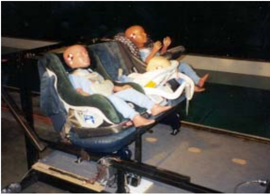
Figure 3. Test sled with three CRS mounted
