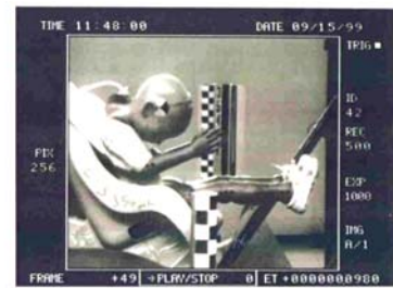
Figure 4. CMVSS 213 Testing of subject seats
