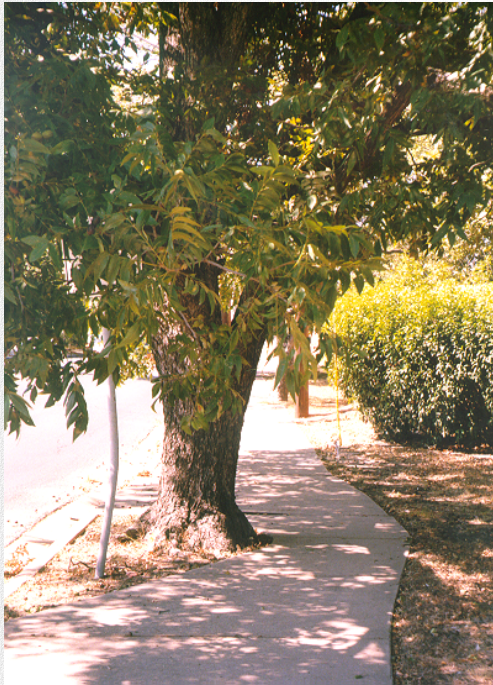
Figure 4-40. If tree roots cannot be removed, the sidewalk should be rerouted around the tree.
