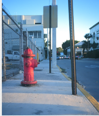
Figure 4-3. Permanent obstacles, such as fire hydrants and street signs, should be relocated to improve a narrow sidewalk.
