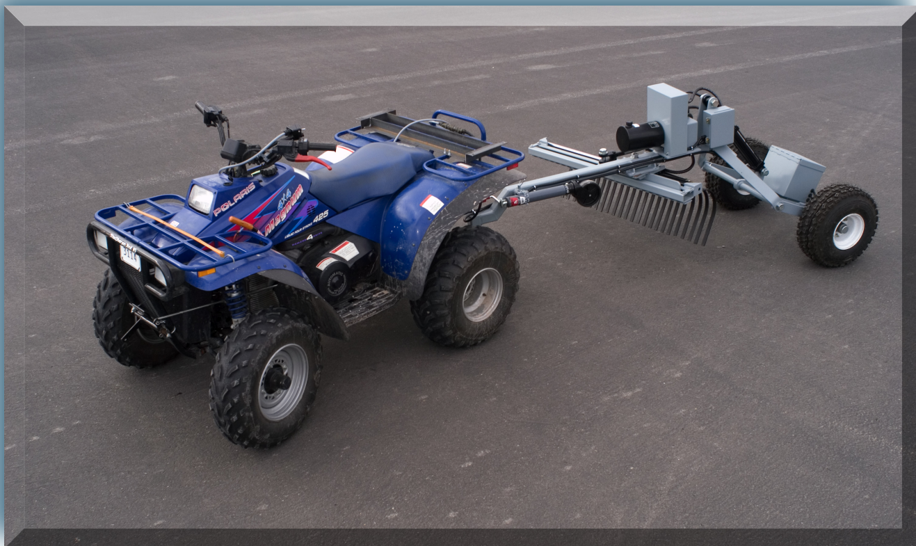
Figure 1—The redesigned MTDC Trail Rake is easier to operate than the original model and can pull dirt back from berms beside the trail without requiring the operator to drive off the trail.
