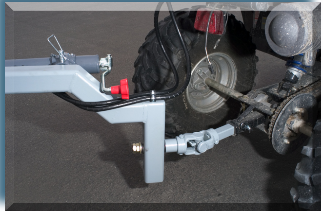
Figure 4—The U-joint assembly connecting the ATV and the trail rake provides better articulation than a ball-and-socket hitch. The receiver on this ATV is custom built. Aftermarket receivers for some ATVs are commercially available.
