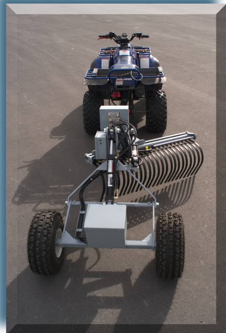
Figure 3—The assembly can be extended 11 inches beyond the edge of the wheels to pull dirt back onto the trail.
