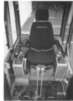
Feature packed operator's compartment with fully adjustable suspension seat, roll back front window, tinted glass, heater, defroster, windshield wiper/washer, AM/FM cassette radio, hand and foot operated travel levers and joystick servo controls.
