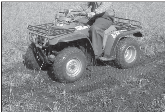
Figure 26—A section of rubber antifatigue mat undergoing preliminary field trials at the Palmer Hay Flats State Game Refuge in Alaska. The large panels install quickly, but the rubber's flexibility limits the panels' ability to transfer lateral loads.
