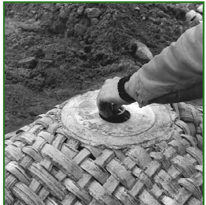
Figure 7—The "primer" cartridge is placed in the breech block.
