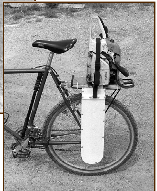
Figure 3—The power head cushion topped with sheet aluminum needs to be high enough so that the saw dogs clear the side scabbard. The height will vary with different brands of saws.
