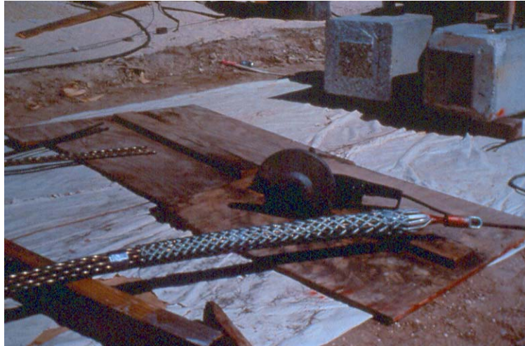
Figure 3.25 – Steel wire sock for installing multi-strand tendon
