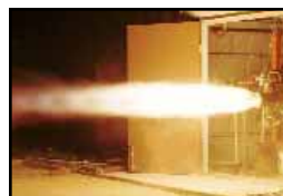
XCOR 5,000 pound-thrust LOX/kerosene engine
