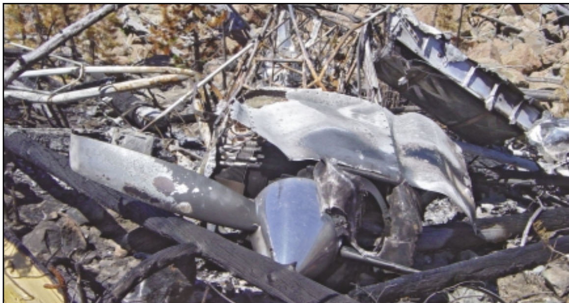
The engine, propeller, and cowling are among the few portions of the aircraft that remain easily identifiable. U.S. Forest Service Photo courtesy of the Helena Flight Standards District Office.
