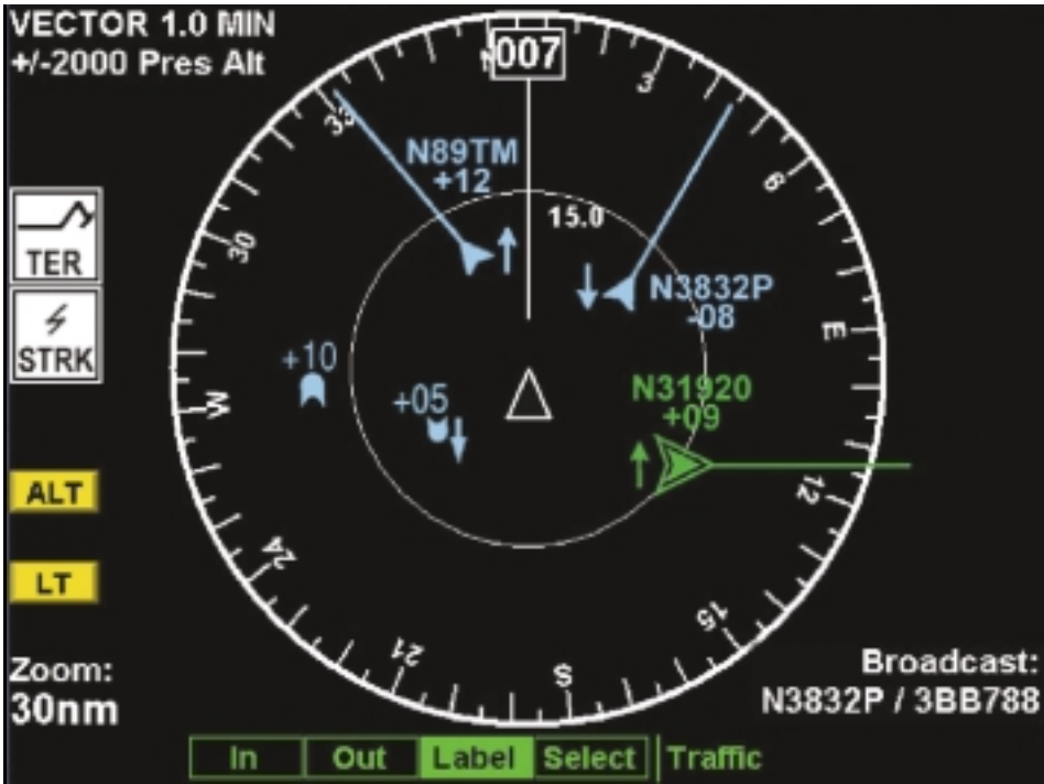
A cockpit display of traffic information (CDTI) showing ADS-B traffic information. Photo courtesy of Garmin.
