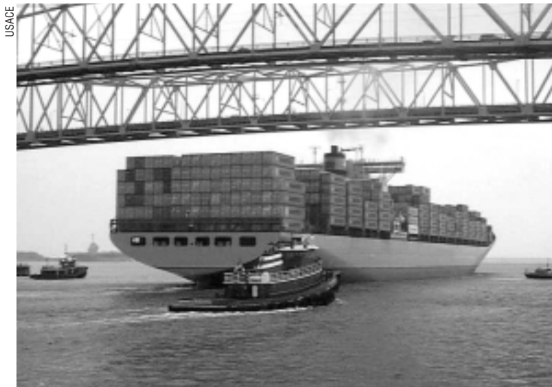
Stacked high with containers, a containership is pushed through Charleston Harbor, Charleston, South Carolina. Containers are measured in twenty-foot equivalent units (TEUs)—the total length of the container divided by 20. A 48-foot container equals 2.4 TEUs.
