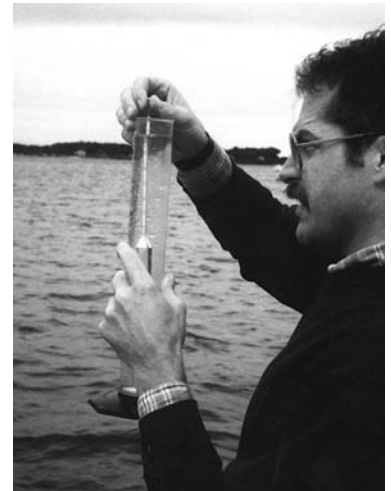
Using a hydrometer. (photo by P. Bergstrom).
