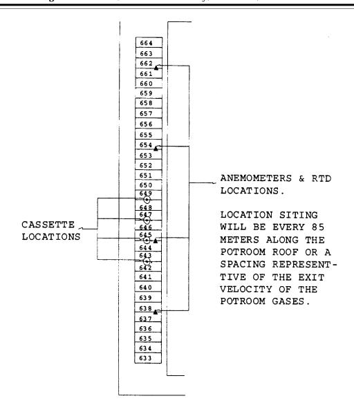
Figure 14A-3. Conceptual side view of positions of cassettes, anemometers, and RTDs in a typical half of a potroom.
