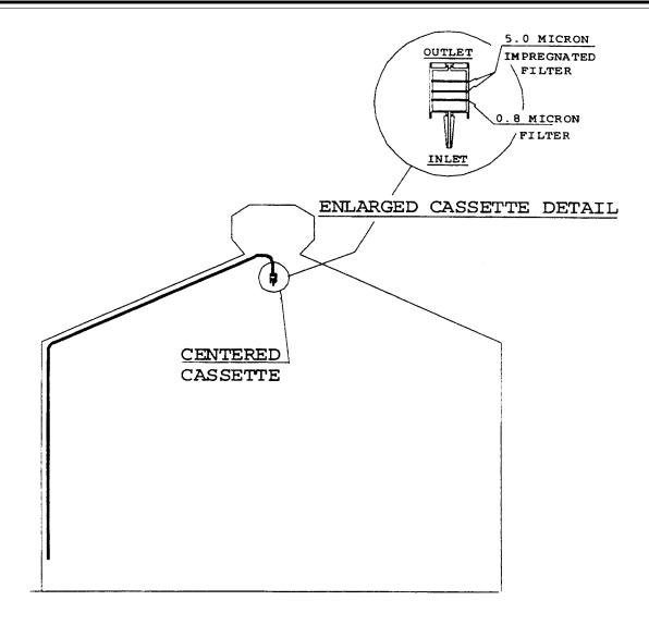
Figure 14A-2. Conceptual end view of cassette placement in a potroom roof.
