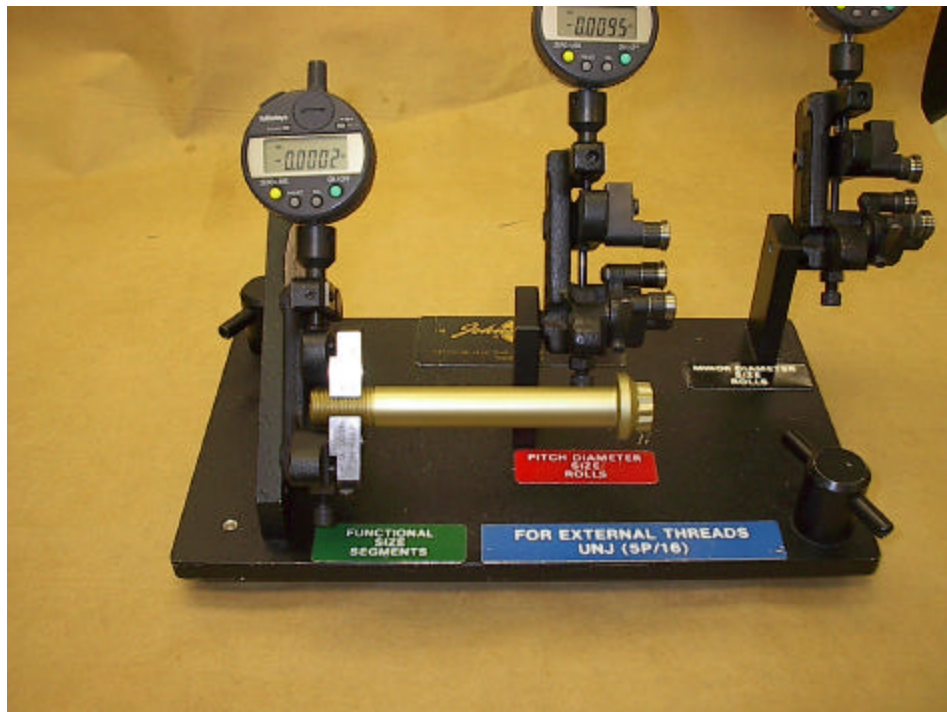
Figure 11 INSPECTION FOR FUNCTIONAL DIAMETER SIZE, FULL FORM SEGMENT INDICATING GAGE
