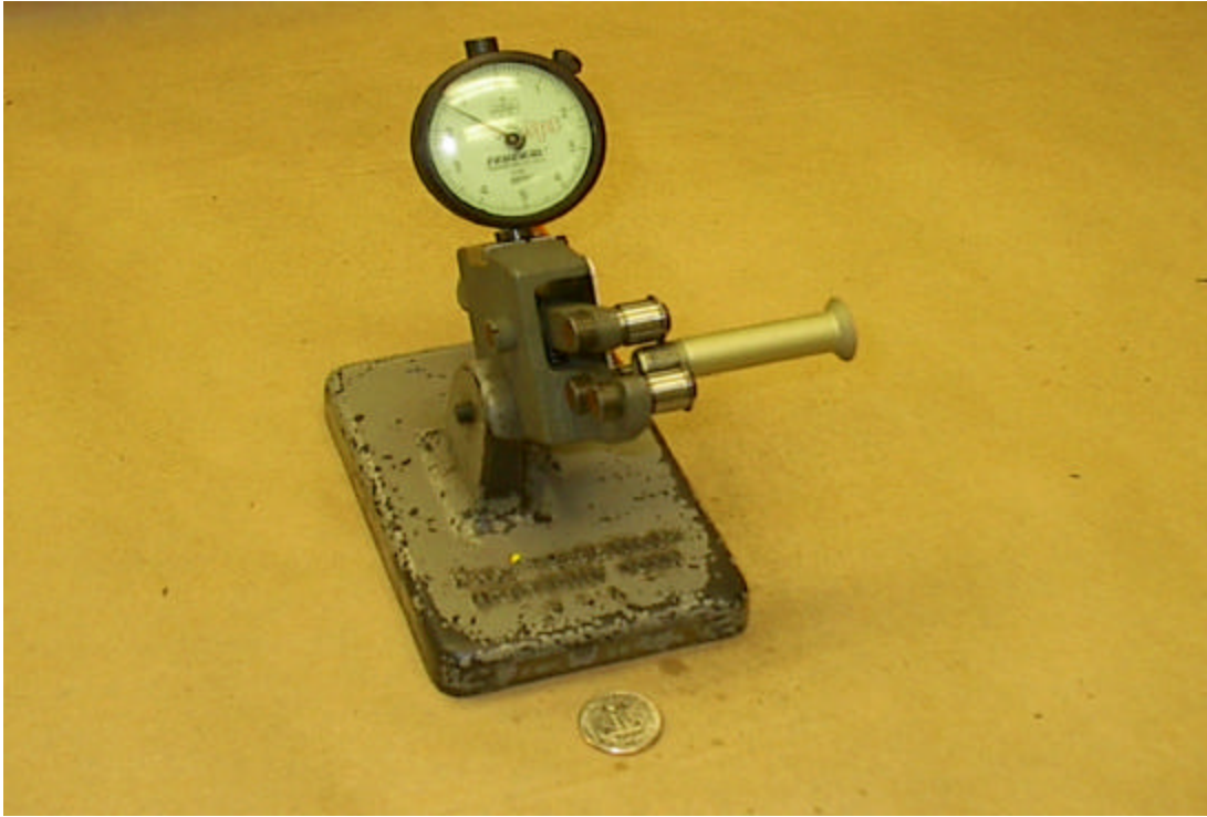
Figure 4 FAA GAGES, THREAD GROOVE DIAMETER (CONE ONLY) TYPE INDICATING GAGE
