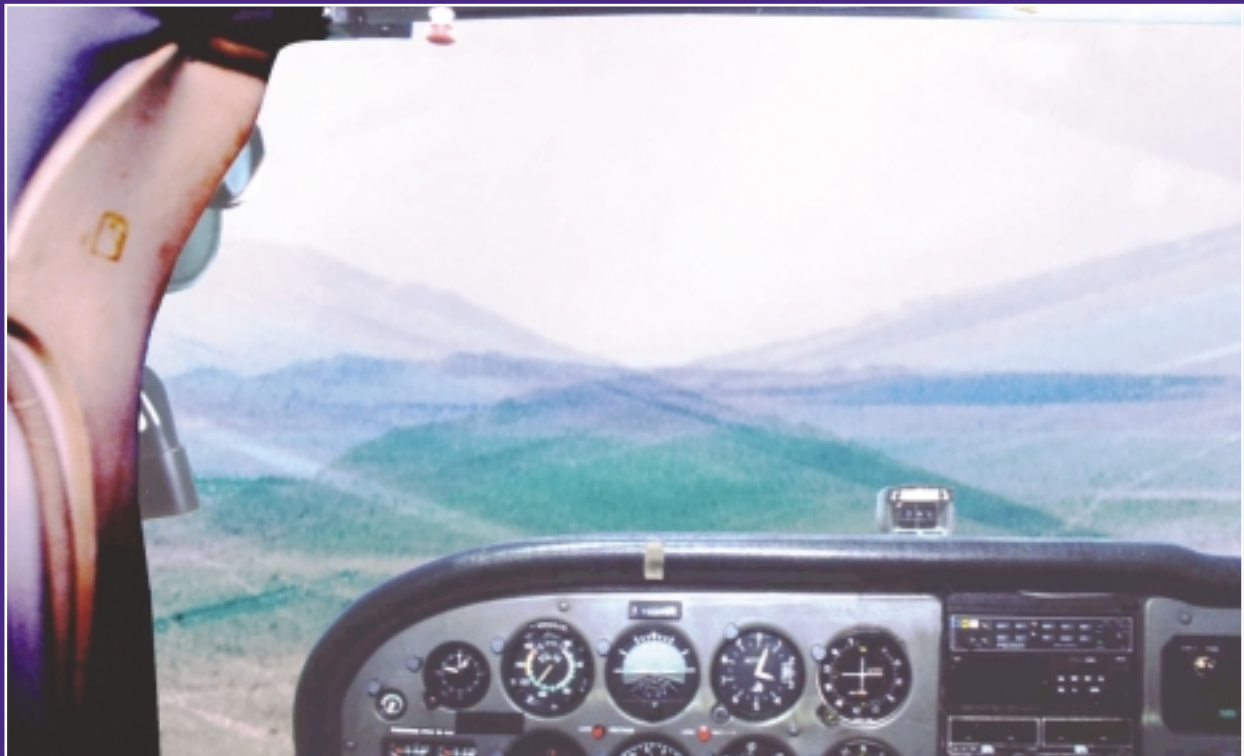
Student's view of rotating the horizon about a point on the windshield
