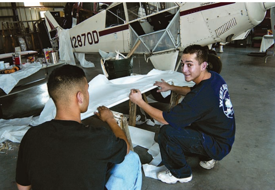
High school students learn fabric recovering thanks to the Thomas Wathen Foundation at historic Flabob Airport in Riverside, California.
