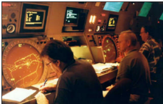
Controllers at terminal radar approach control facilities provide guidance to pilots as they enter and leave the immediate area of the airport.
