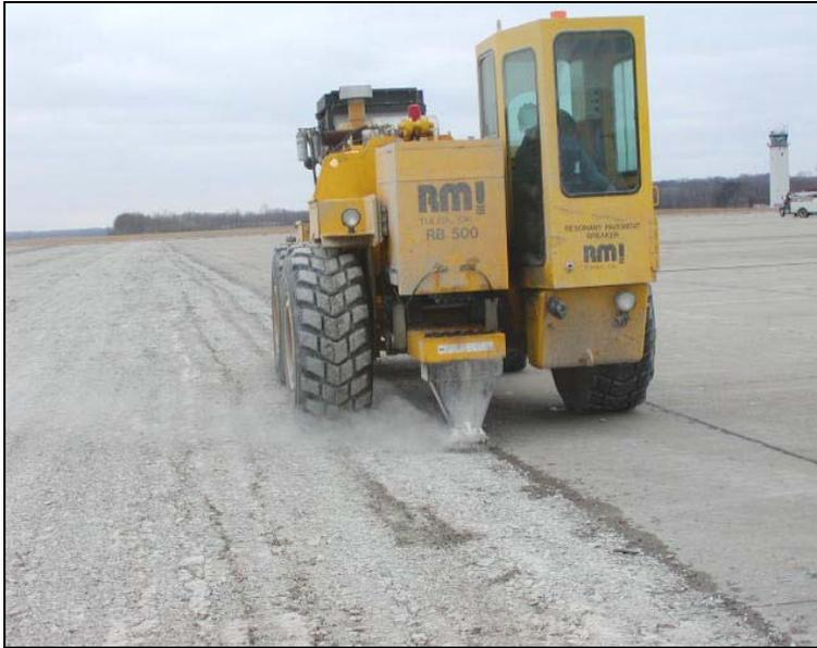
**Figure 1. Resonant Breaker Machine**
