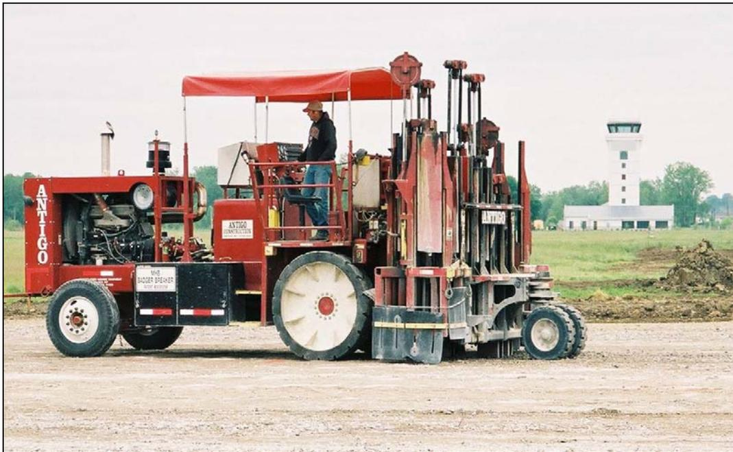
**Figure 2. Multi-Head Breaker Machine**
