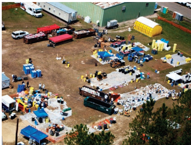
Following Hurricane Katrina, EPA collected household hazardous wastes at a central facility in St. Tammany Parish, Louisiana. EPA identified the wastes, categorized and separated the containers, and then consolidated the wastes for transport to recycling, treatment or disposal facilities.
