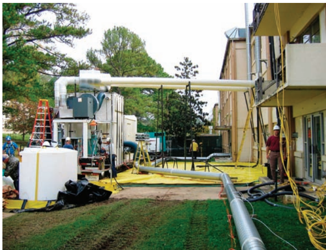
EPA directs field activities during testing of a portable chlorine dioxide generation system that could be used to decontaminate small, indoor areas after an indoor anthrax spore release. EPA collaborated with the Department of Defense to carry out the field tests.
