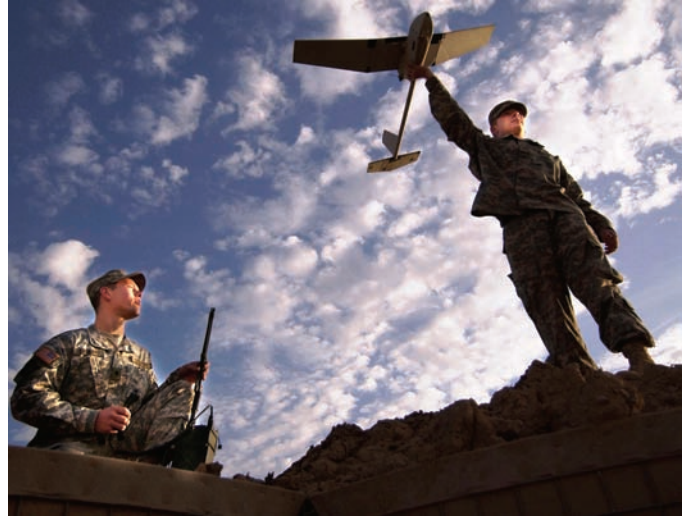
Soldiers from the 101st Airborne Division prepare to launch the Raven unmanned aerial vehicle at Forward Operating Base McHenry, Iraq. The Raven is being used to hunt for roadside bombs.
